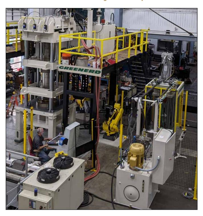
Greenerd Press & Machine Company has announced it has designed, engineered, built and turnkey-installed an automated two-press, two-robot production cell enabling unattended production of large aluminum pressure vessels.
