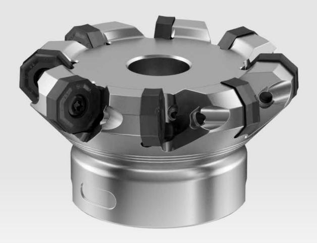
For the utmost in milling productivity, the CERATIZIT MaxiMill 273 Shell Face Milling Cutter provides 16 useable, axially adjustable cutting edges that allow for higher feed rates and guarantee exceptional surface finishes. The MaxiMill 273 is part of CERATIZIT's line of indexable milling cutters that provide quality and flexibility for all milling operations, whether face milling, shoulder milling or high-feed milling.
